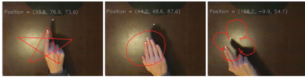
Figure 10: Different shapes drawn using different hand gestures with a single interaction point. Shapes can be drawn by connecting multiple contact points with line segments (left), or by a continuous finger motion (middle and right).
