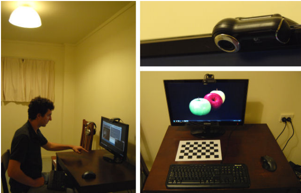
Figure 8: The virtual touch screen set-up employed during development. Left: The positions of the point light source, desk and camera. Right-bottom: The interaction surface (desk) with camera and calibration grid. Right-top: The orientation of the camera with respect to the monitor and desk.
