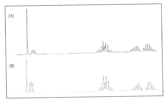
Diagram 2.7: 'H NMR of the observed spectrum (A) and the simulated spectrum (B) of [Pt(L-glu.OMe)Cl<sub>2</sub>]<sup>-</sup> at 300 MHz.
