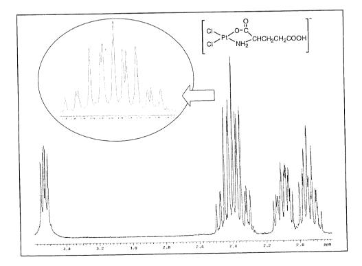
Diagram 2.6: 'H NMR of [Pt(L-glu-N,O)Cl<sub>2</sub>]<sup>-</sup>.
