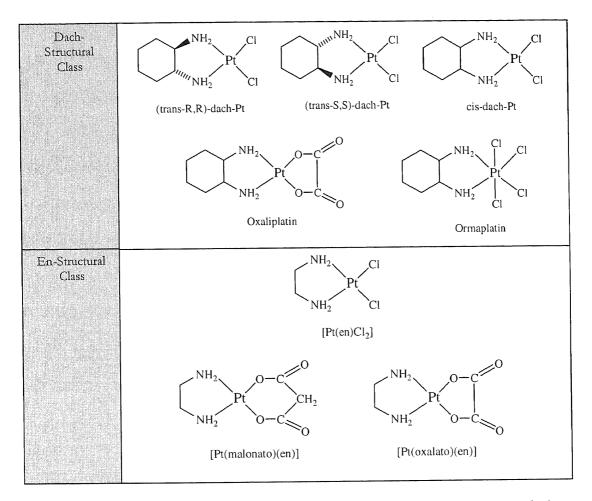
Diagram 3.3: Chemical structures of the common platinum compounds containing dach or en.
