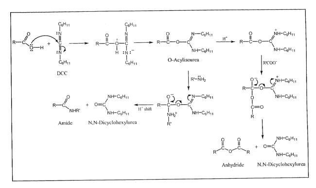
Diagram 6.2: Reactions of DCC with carboxylic acids.
