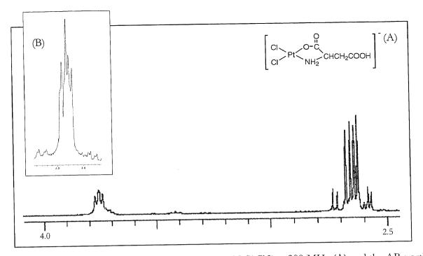
Diagram 2.4: The 'H NMR spectrum of [Pt(L-asp-N,O)Cl<sub>2</sub>]<sup>-</sup> at 300 MHz (A) and the AB-portion at 200MHz (B).
