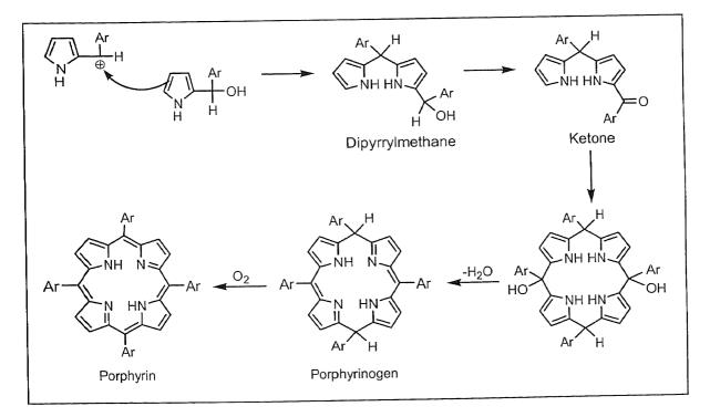
Diagram 5.3: Mechanism of TPP synthesis
