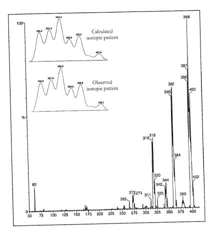
Diagram 2.11: Mass spectra of [Pt(L-asp-N,O)Cl<sub>2</sub>]<sup>-</sup>
