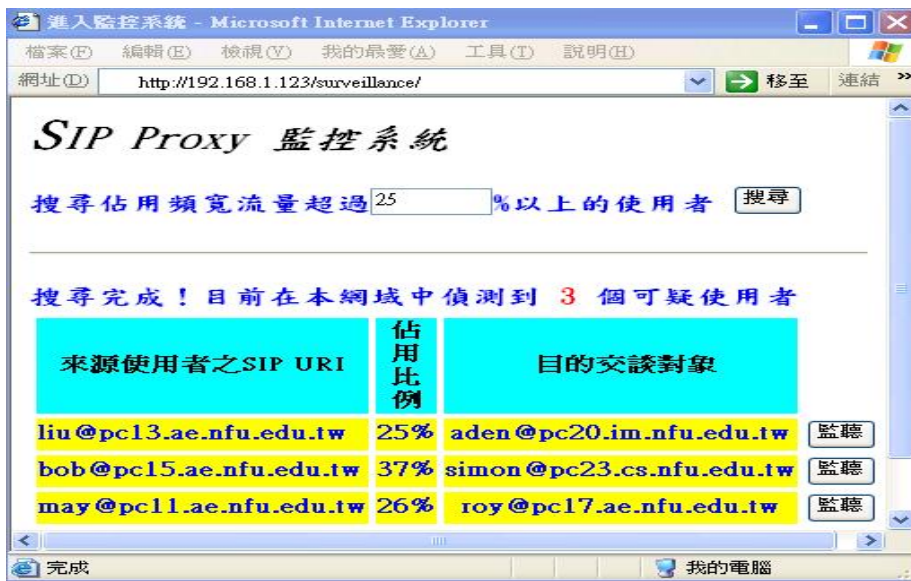
Figure 7. The requested user information provided by the SIP server through the web server.
