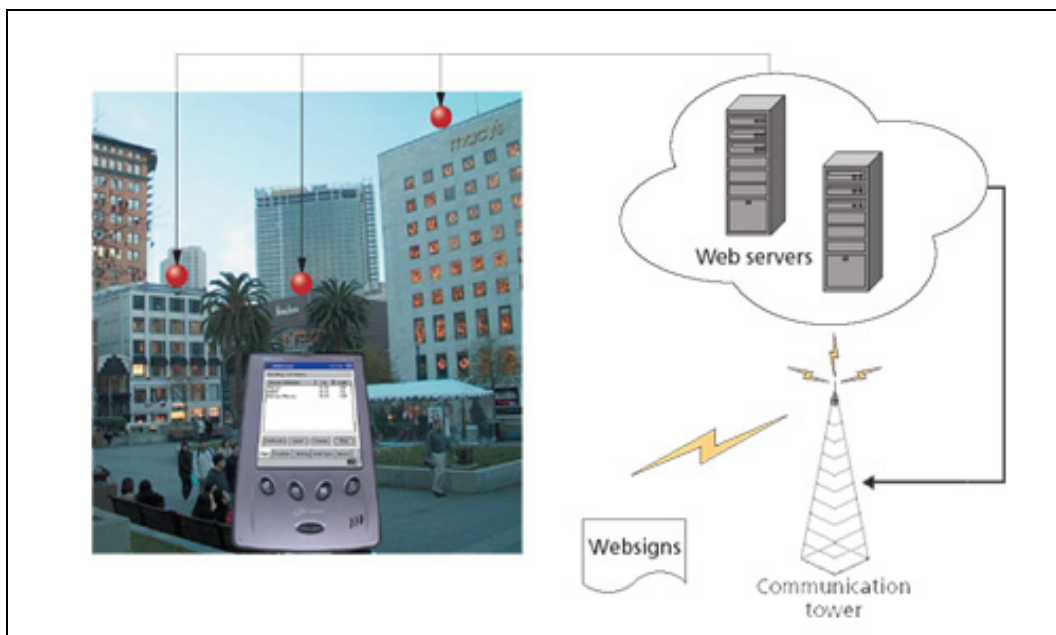
Figure 2: Example of a “websign”: Web servers detecting websigns with a wireless PDA in an urban environment (Source: Pradhan et al. 2001)
