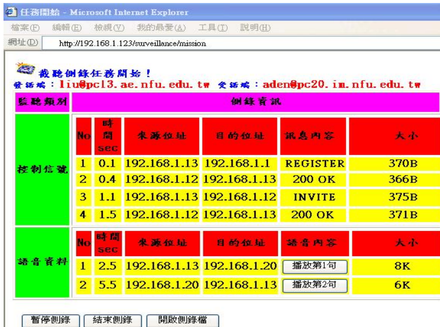
Figure 8. The interception and wiretapping data after retrieval from the SIP server and display to the agent through the interactive web server.
