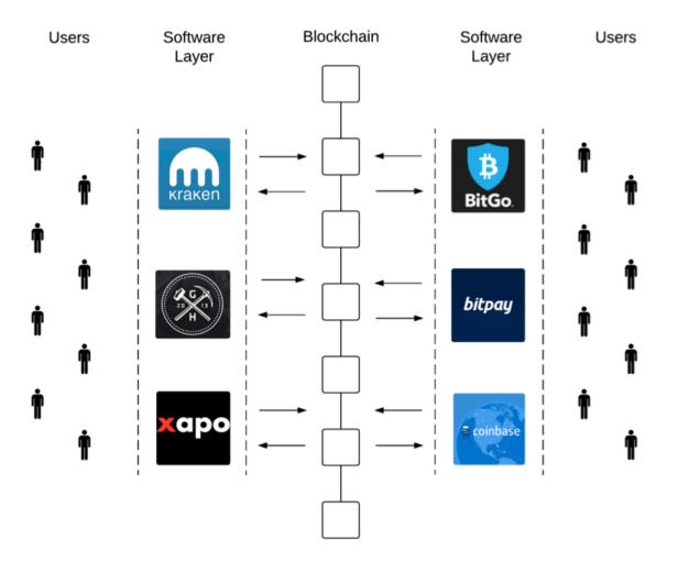
Figure 36: Layers of software built on top of the Bitcoin blockchain that interact with the protocol on their customers' behalf creating channels (or bottlenecks) of user activity
