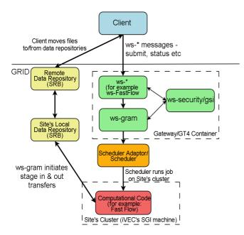
Figure 1. Geosciences Grid SOA architecture
